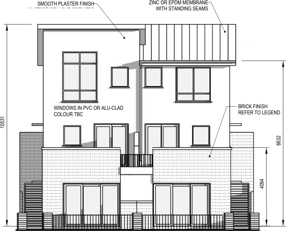
FRONT ELEVATION [TYPE M] SCALE 1:100
